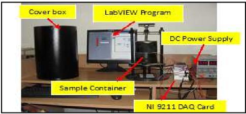
Figure No.1: Experimental setup for transient heat plane source
