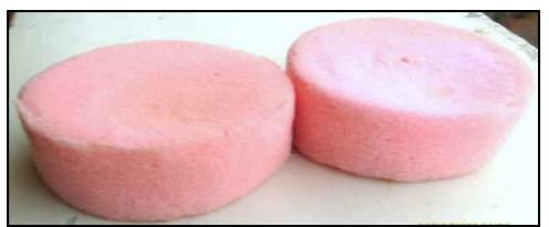
Figure No.2: Polyurethane Foam Sample
